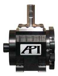
SwivelCheck utilizes a servo-drive to calibrate rotary axis and rotary and tilt tables integral to the machine tool calibration process.
